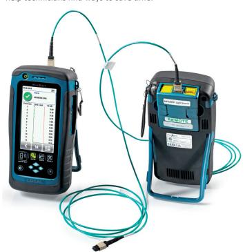
The ability to choose from a range of interchangeable adapters, like these, helps distribute device cost across less-expensive components. Copper, singlemode, and multimode adapters easily plug into and out of the unit.
